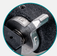
Torque set at CCW/CW control via double throw switch on operating button.
